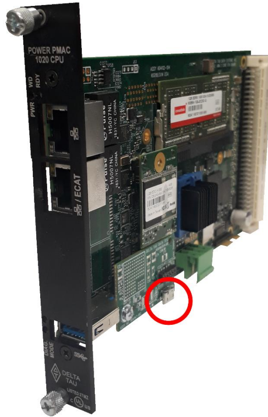
Figure 2. USB Connector is for a mass storage device
